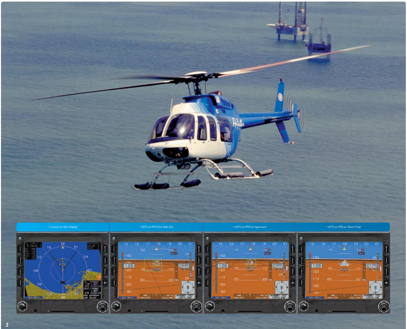
3 The screens inset in the photo above illustrate how Highway-In-The-Sky (HITS) makes flying to any spot on the face of the earth simple. The nav display on the the Multi-Function Display (MFD) shows your overall course. On the Primary Flight Display (PFD), the green HITS boxes lead you unerringly to the landing pad on an oil platform, a rooftop, or any lat/lon or radial/distance point you choose. Highway-In-The-Sky is also ideal for water search and rescue. You can easily program a search grid that blankets a sector and then fly it with unerring accuracy to ensure that no area within the sector is missed.
