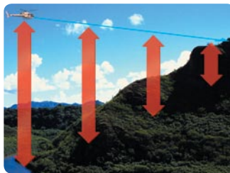
Excessive Closure to Terrain
