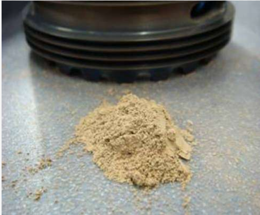
Photo 1: This engine was typical for a NZ operator without a filter – about 6 grams of dust after 1200 hours
