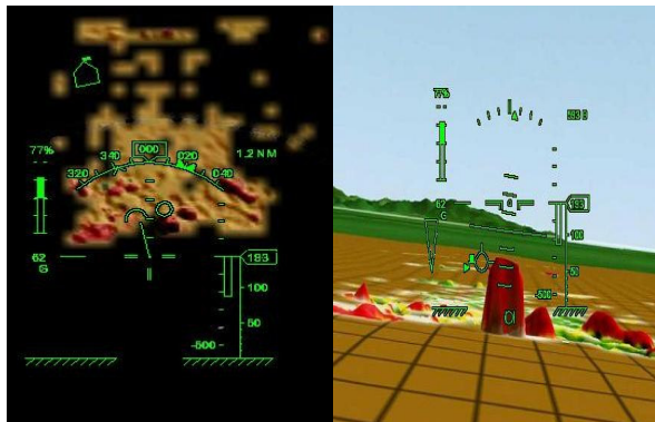
Figure 7: BLAST synthetic vision image in plan view (HSD) and egocentric 3-D view (VSD) with BOSS overlay
