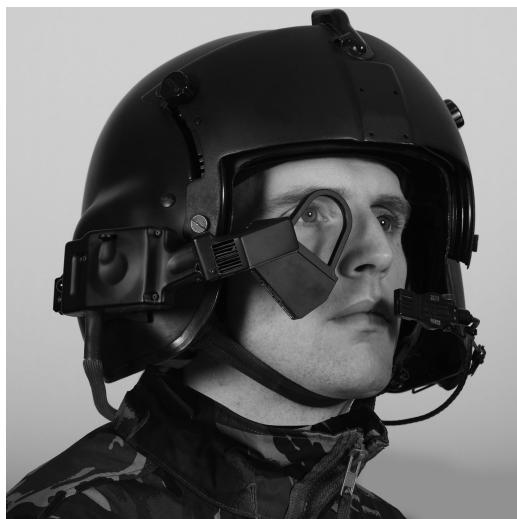
Figure 5: The BAE Systems Q-Sight™ 150 helmet mounted display
