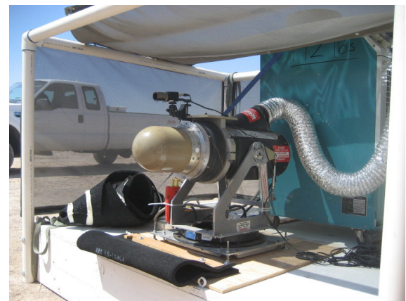
Figure 16: Sensor, sensor mounting tube, gimbal, and ambient forced air
