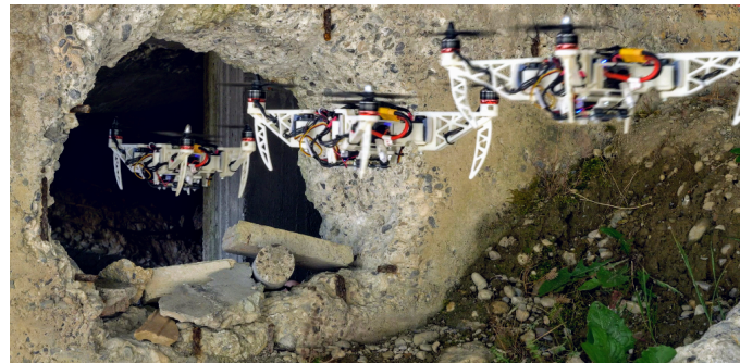
Fig. 1: Quadrotor with morphofunctional folding capabilities. The drone can transition from the standard X configuration to task-specific morphologies: (a) H configuration to fly through narrow vertical gaps; (b) O configuration, where the drone is fully folded to fly through horizontal gaps; (c) T configuration for proximity inspection of vertical surfaces. (d) Traverse of a gap narrower than the vehicle size using the H morphology. From right to left: the quadrotor approaches the gap with the X configuration; the vehicle initiates the folding maneuver to reach the H configuration; the gap is traversed using an elongated morphology to avoid collisions.
