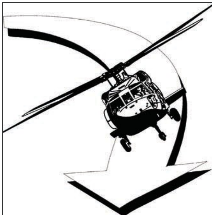
Figure 4-2. Centripetal (radial) acceleration
